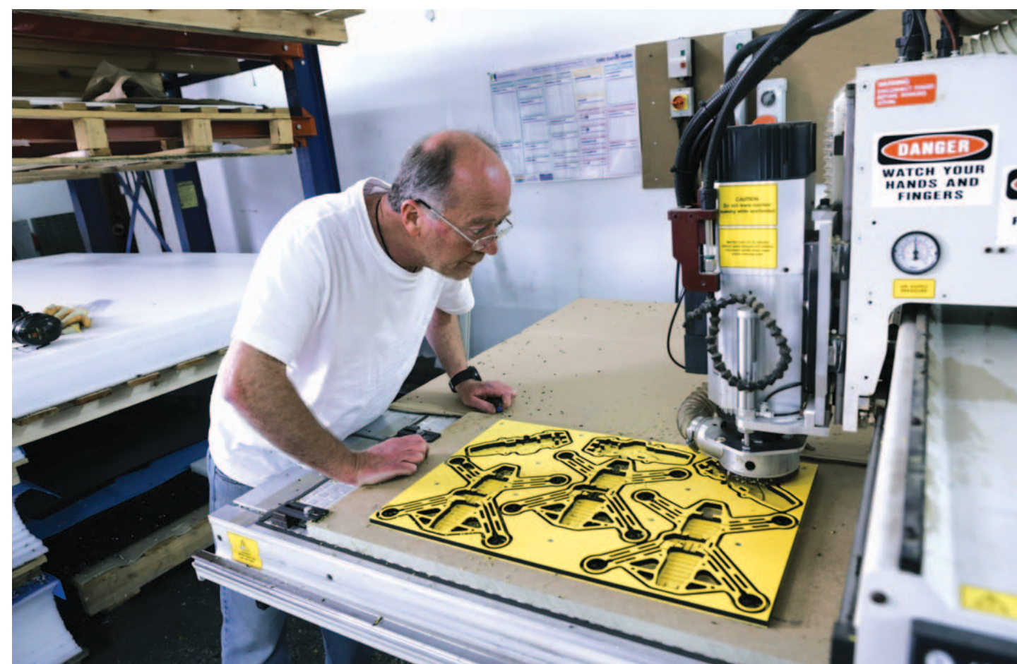
Martin Rye, owner of Fossils Stuff, watches closely as his CNC machine cuts Gravity 280 frames.
