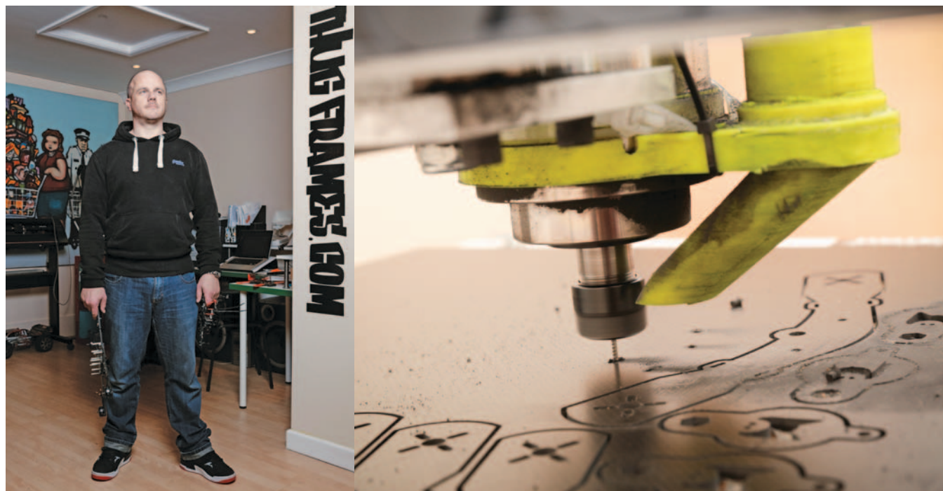
Left: Stefan Mirfin at the Thug Frames studio in Kent, England. Mirfin recently relocated to give his workshop and equipment more room to meet the growing demand. Right: Thug Frames' specialist CNC machines cut carbon-fiber frame parts 24 hours a day.
