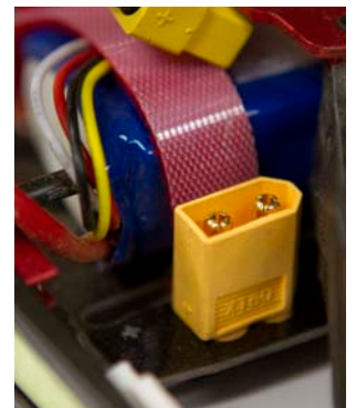
Below right: A nice design is having this power plug attached to the body, making an easy and solid electrical connection.
