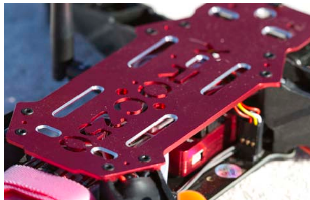
Left: The solid-metal chassis on both the top and bottom gives this quad enhanced protection from hits and bumps, and it has a great look to it.
