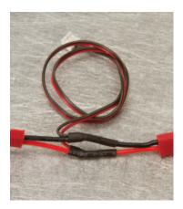
Spektrum Air Telemetry Flight Pack Voltage Sensor
